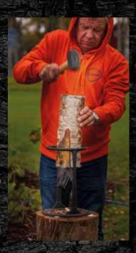
A safe and easy-to-use way to split firewood into kindling. Kindling Cracker is durable, because it is made out of one single piece of cast iron, and brushing is normally the only maintenance it needs.
